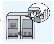
\*Cabinets: By attaching an earthquake resistant latch to a cabinet, you can prevent injuries and further damage to your house.
